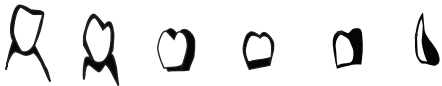
Modified Socket Porcelain Butt Margin Full Metal Collar (360) Metal Occlusal Metal Lingual
